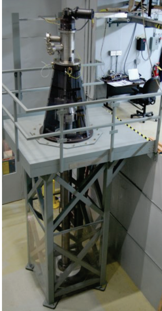
Figure 4.40. ORNL rotating target mock-up testing.
