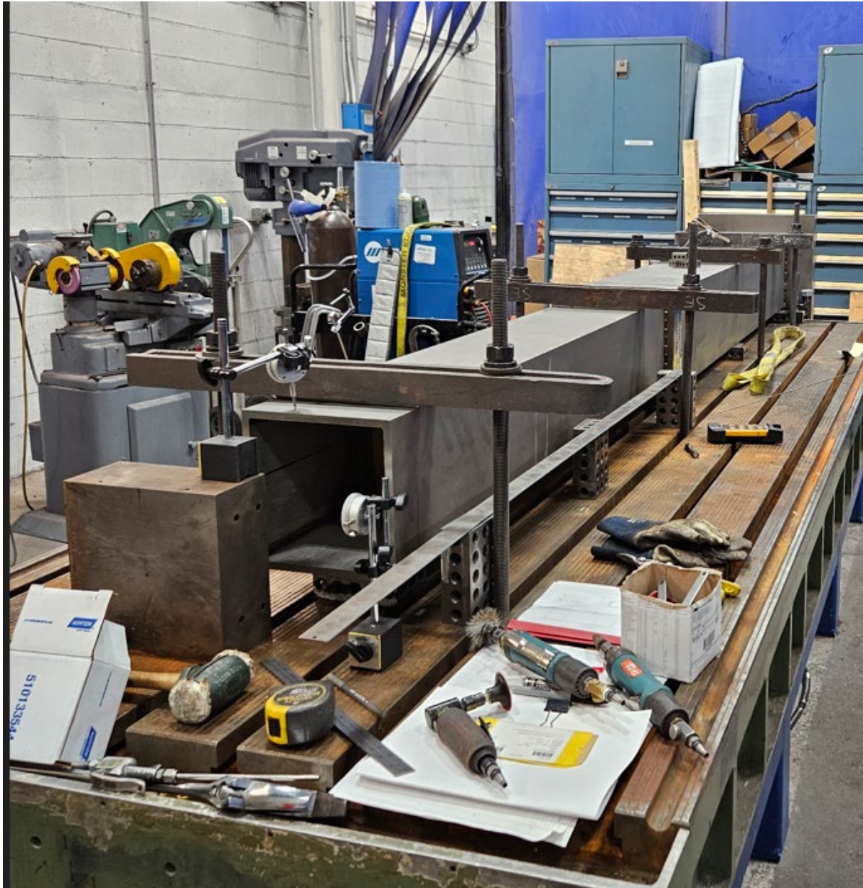
Figure 118: Prototype Nozzle Extension during fabrication at Keller Technology Corporation
