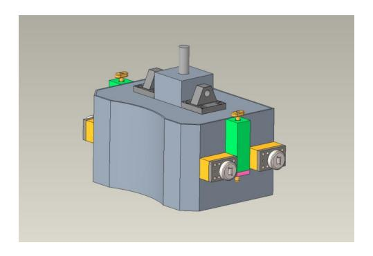
0.5-Inch-Thick Stainless-Steel Vessel 30 cm of lead thickness ~850 kg vessel mass
