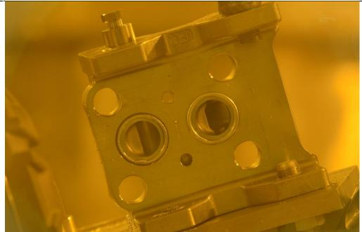
This supports the conclusion that the cause of the mercury leak is corrosion of the silver-plated Inconel X-750 process seals. These seals are present in the Rosemount 3145N sensors, including both P-5001 sensors that were installed during this run cycle. Due to this, it would be expected that the second of the P-5001 sensors would develop a leak soon if returned to service.
