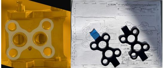
The sensors were repaired by removing the silver-plated seals, and re-assembling generally per Rosemount Reference Manual 00809-0100-4835 Rev BG, Page 63, except using the gasket in place of the process C-rings, and not using torque tools to measure the applied torque. The seals were then pressure tested to verify assembly. See 106070100-WKI10010 for more details of the assembly and testing process.
