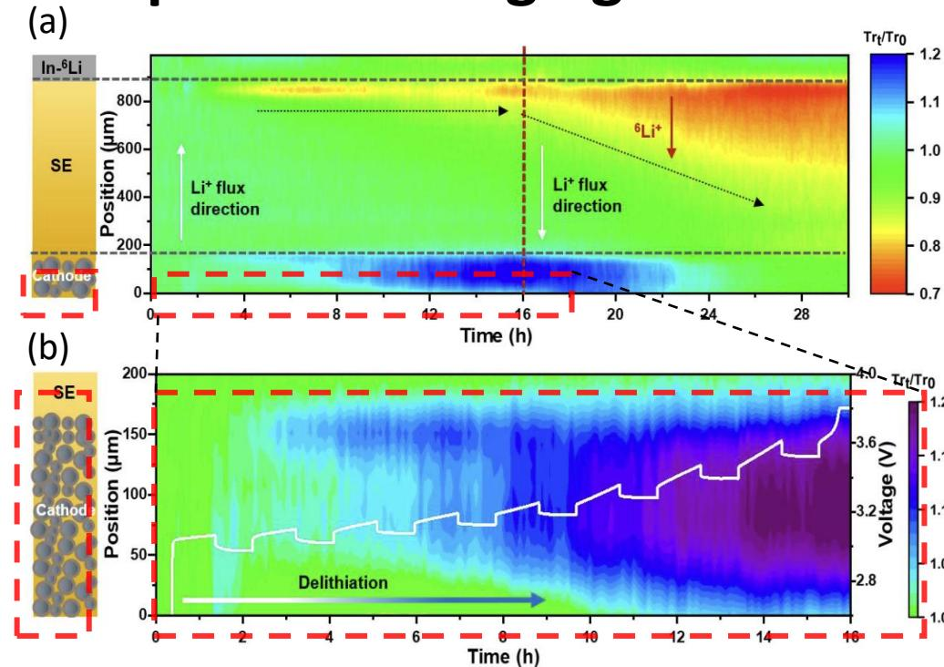
(a) Position vs. time plots with the averaged neutron transmission (trans.) changes ( $Tr_t/Tr_0$ ) represented in color.  $Tr_t/Tr_0 < 1$  indicates reduced trans. due to Li increase or  $^{nat}Li$  replaced by  $^6Li$ ,  $Tr_t/Tr_0 > 1$  indicates increased trans. due to delithiation.
