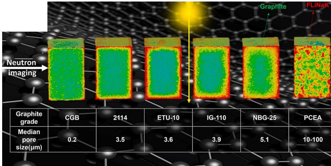
Neutron tomography results for selected graphite grade in this study. Virtual cut has been applied at the center to expose the internal salt distribution (blue/green: low salt conc., yellow/red: high salt conc.). The median pore size and graphite grade is listed in the table. FLiNaK salt intrusion was conducted at 750 °C, 5 bar for 12 hrs.
