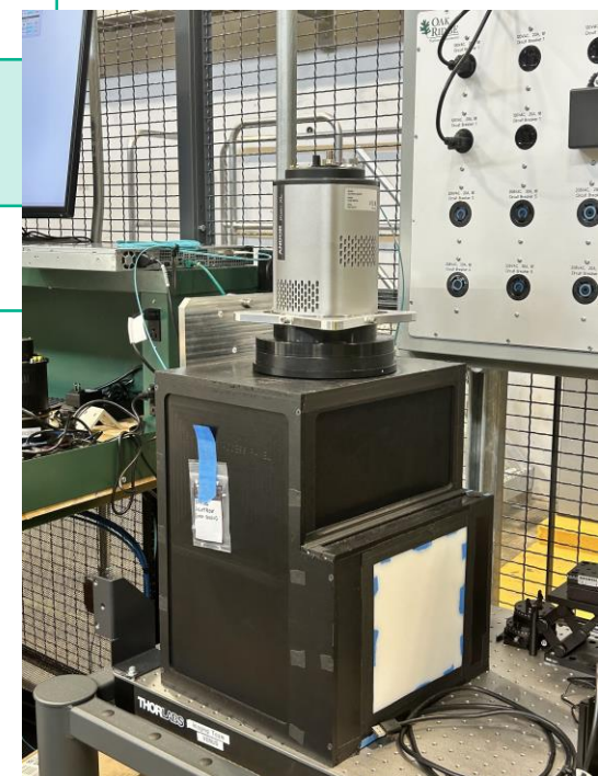
ANDOR iKon-XL CCD mounted on 20x-20 cm 2 light-tight box
