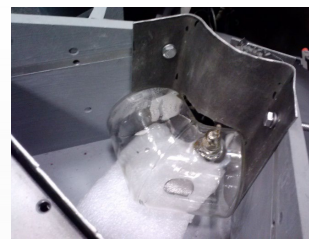
Thanks to NCNR for providing wide angle 'banana' 3He cell for ORNL
