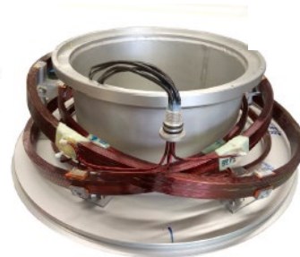
2 pairs of compensated Helmholtz coils, tilted to produce guide-field in the YZ plane
