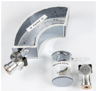
Banana type analyzer cells with Si-windows
