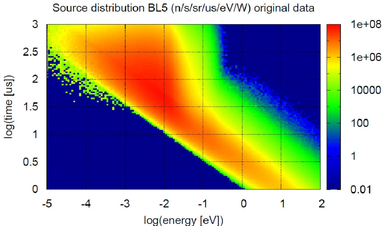
Fig. 12: Short-pulse emission time distributions for the coupled top downstream SNS hydrogen moderator on linear (at top) and logarithmic (at bottom) scale as simulated by Wei Lu with MCNPX [2].
