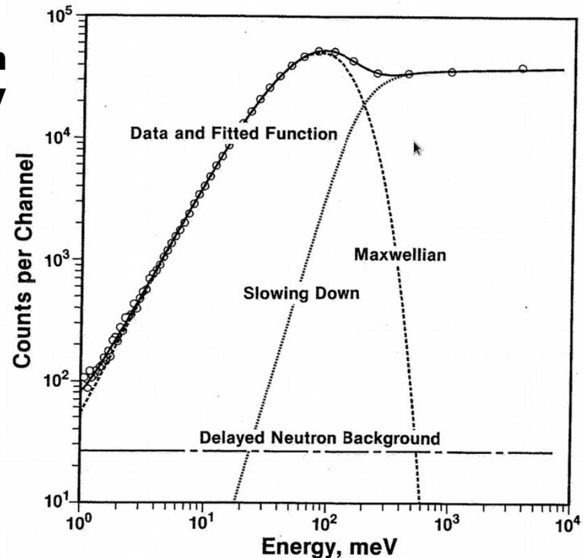
FIG. 35. The counting rate in a  $1/v$  detector, proportional to the beam current per unit lethargy  $Ei(E)$ , for a heavily irradiated ambient-temperature polyethylene moderator. The
