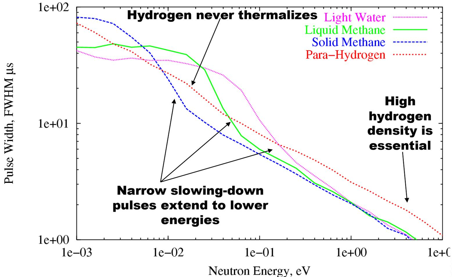
**Intensity / FWHM<sup>2</sup> at 20 meV is best for coldest moderator, where the pulse width is still in slowing-down behavior, even though it's 5x less intensity**
