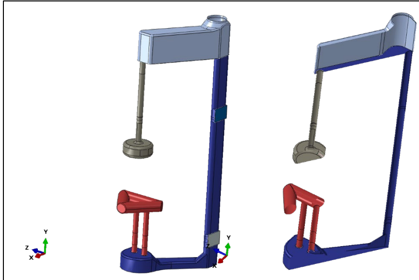
Figure 45 Vacuum Boundary Surface
