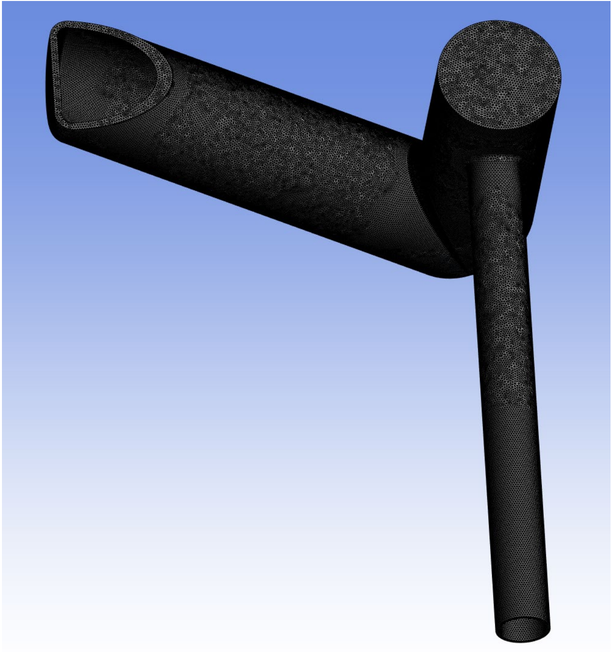
Figure 5.4 Lower Hydrogen Vessel Refined Mesh
