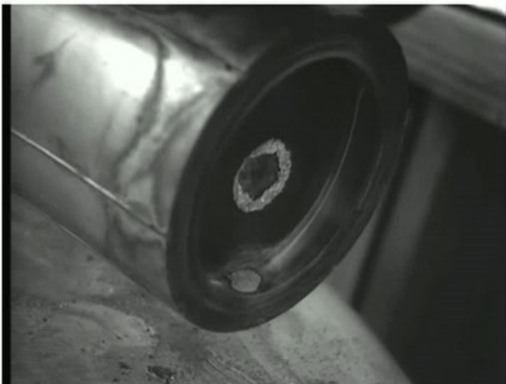
Figure 3-3 ISIS TS2 tantalum window failure
