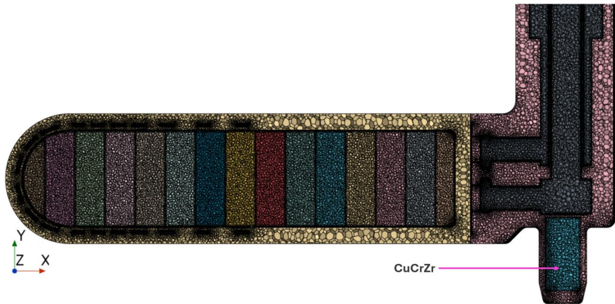
Figure 13. Section view of the mesh configuration for the target segment.
